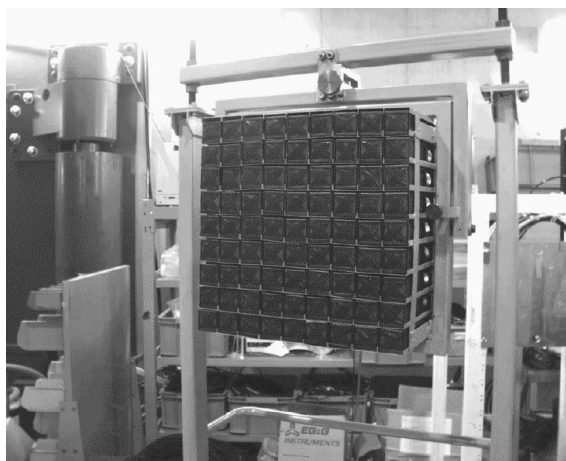
Figure 1: A view of the neutron array detector built within the cooperation agreement between the NIPNE, Romania and RIKEN, Japan. It consists of 81 detectors made of 4 \times 4 \times 12 \text{ cm}^3 BC-400 crystals, mounted on XP2972 phototubes.
